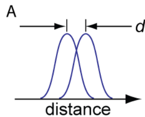
Figure 2: Resolution of an imaging system is based on the observation of its PSF. The smallest distance that can be discerned is given by d (see text). Since the PSF is narrower along the lateral direction than along the axial direction, the lateral resolution is higher than axial resolution. See Fig. 1 for details.
