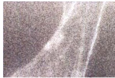
Figure 5: Crossover effects contribute to noise level (i.e. poor SNR), as shown at right.
