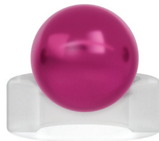
Figure 4. Imperfect seal with ball wedged into the seat ID.
