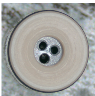
Figure 14. Crystallization in ball cage.
