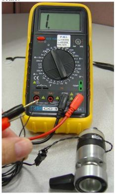
3. Switch the valve to inject. It should now read zero.
