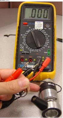
If the reading does not change the switch needs to be replaced.
