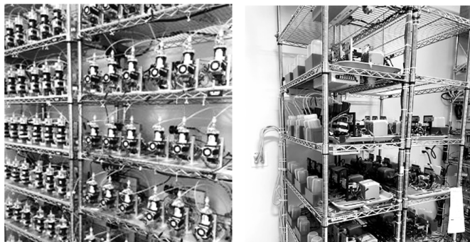
Figure 3. Example of pump testing setups in our Middleboro, MA facility. The left image shows multiple molded head pumps on life test achieving multiple millions of cycles. The right image shows the testing of a durable VFP17-DRB model using high saline and detergent-containing reagents.
